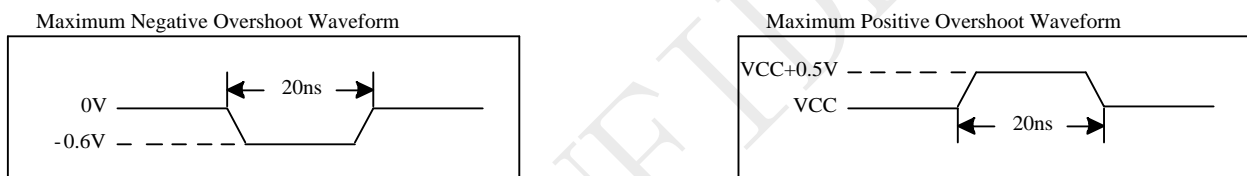
Figure 5-1 Maximum Overshoot Waveform
